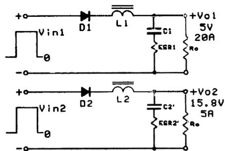
Fig 2 Equivalent Sources
