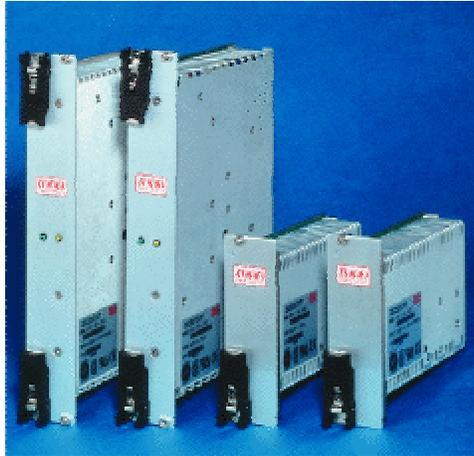
**1. These 150-W CompactPCI supplies conform to the standard's mechanical requirements of 3U or 6U high, 160-mm deep, and 8HP wide. The specification also calls for the use of a DIN "M" connector.**
