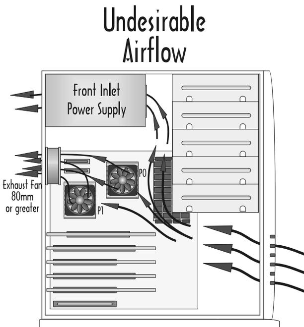
A power supply with a front air inlet causes a portion of the airflow to be diverted directly through the power supply, never passing near the heatsinks. With this type of power supply, there is a greater potential for overheating problems.
