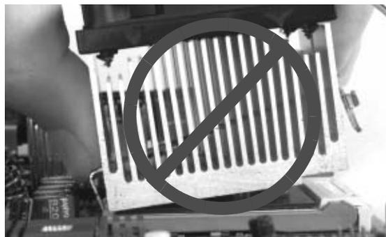
Photo 7. Wrong way to install heatsink
