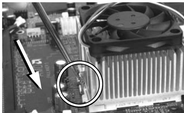
Photo 10. Push clip down and in to fasten
