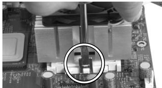
Photo 11. Always keep clip aligned with lug
