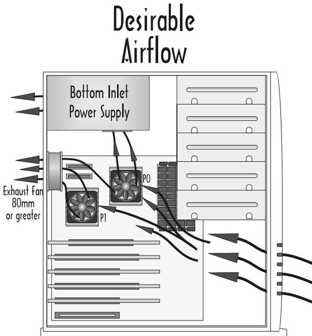
Testing by the AMD thermal engineers has shown that the airflow pattern seen in Figure 1 is more desirable than the airflow pattern seen in Figure 2. When the bottom inlet power supply is used, nearly all the air flows near or through the area of the processors. As a result of this, the processors remain cooler. Since the heatsinks are heat radiators, like the radiator in your automobile, they need airflow to function properly. The more airflow there is, the better they function.
